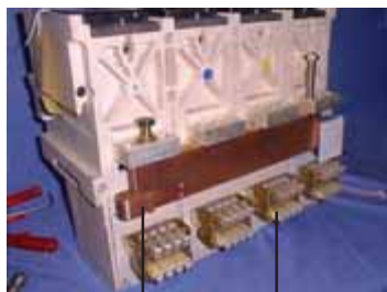
1.Spring loaded earthing contact.
